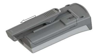
Before attempting clip replacement, ensure that the grip adjustment slider is set to the top of the clip and that the metal back-plate has been straightened. Re-insert the metal clipback into the guides on the case-back and slowly slide the clip assembly into place, ensuring that the retaining lug re-locates into the slot in the case-back.
