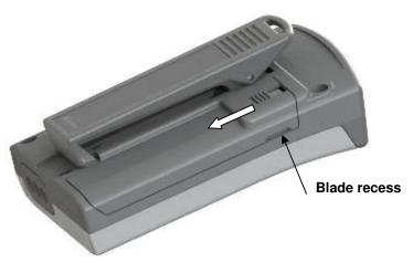
Hold the pager in one hand, with the front facing downwards. Using thumb or forefinger, gently slide the catch in the direction of the arrow shown. Insert a thin blade (e.g. small screwdriver) or finger nail into the recess on the side of the door and gently lift enough to release it from its retaining slot.
