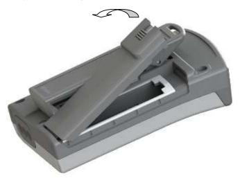
Carefully lift and release the battery door away from the main body in the direction shown, ensuring not to damage the rubber seal around the edge of the battery compartment. Ensure that the battery door is lifted clear of the case and remove the door. Remove the battery by placing your forefinger onto the positive end-cap and lifting the battery upwards, at the same time pushing slightly backwards against the negative contact spring.
