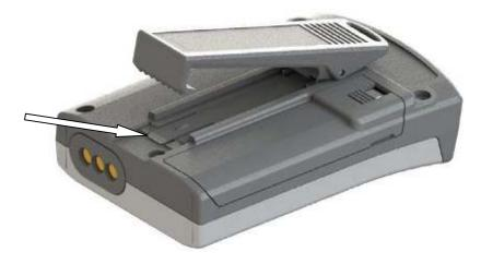
Insert a thin blade or fingernail under the edge of the backplate as indicated by the arrow and lift away from the pager body. Once the plate is clear, gently slide the clip towards the bottom of the pager, until it comes away from the main body.
