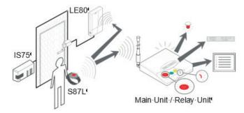
The S87L Wristband Transmitter with Locating function is designed to interact with the following devices:
