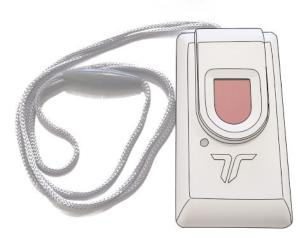
Its compact size, waterproof case and ease of operation make the S35 Pendant Transmitter the perfect solution for use at home with a Carephone. The alarm is triggered by pulling the cord or pressing the red button, releasing a call to the Carephone.
