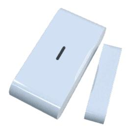
The RAC80 Radio Alarm Contact detects the opening or closing of an electrical contact or of a door equipped with a magnet. This sends a radio warning to a Nurse Call unit. The RAC80 Radio Alarm Contact provides a magnetic reed contact for monitoring doors and windows. The internal reed contact is activated by an external magnet which can be placed in the position indicated.
