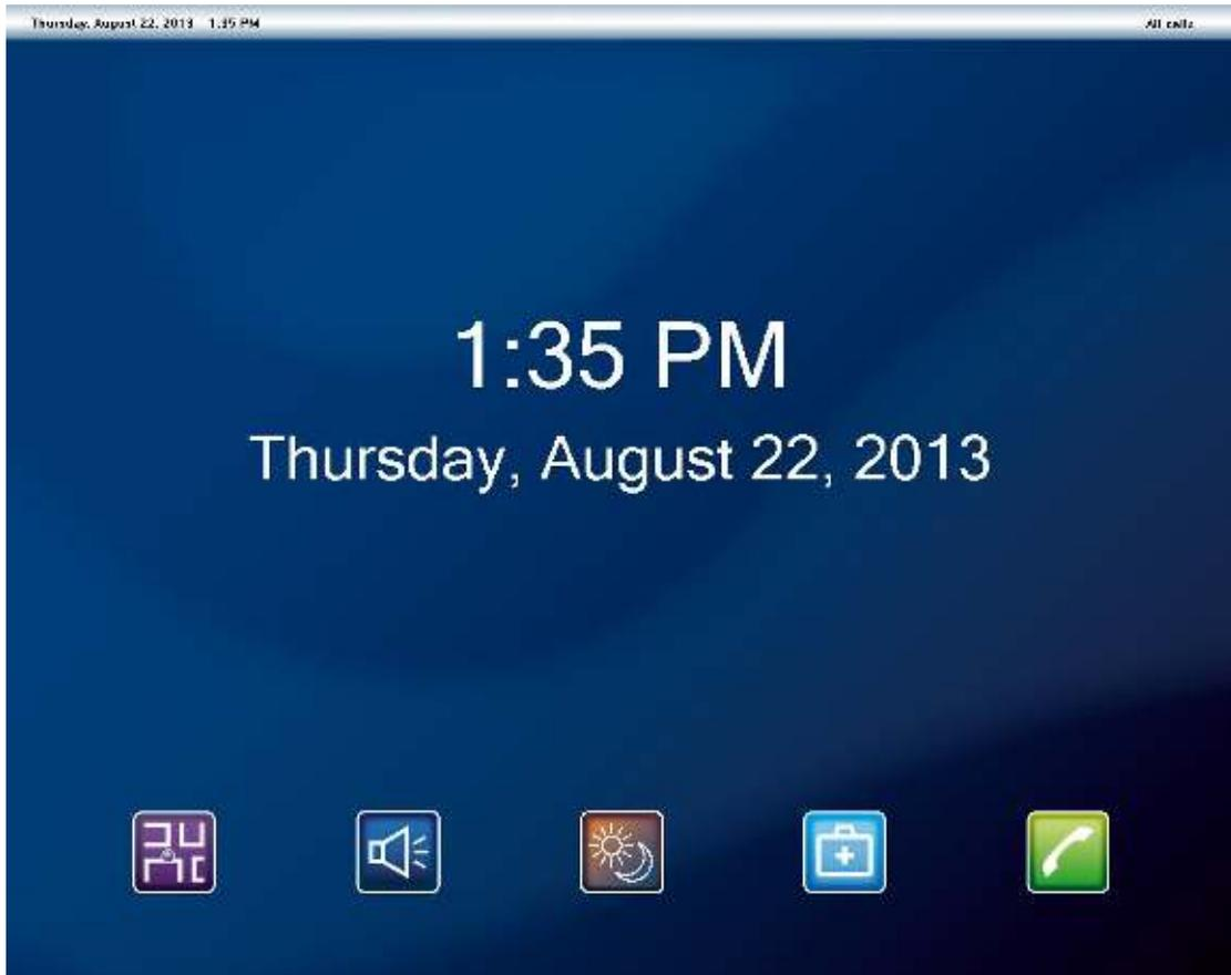
The main screen consists of a 3 parts: A header showing current date and time on the left and the current DN setting on the right. In the middle section the pending calls are shown, or date and time will be displayed when there are no pending calls. At the bottom you find the icons that allows you to change your preferences and settings. The icons can be hidden or set to idle with a password protected activation using the MSPC Manager.
