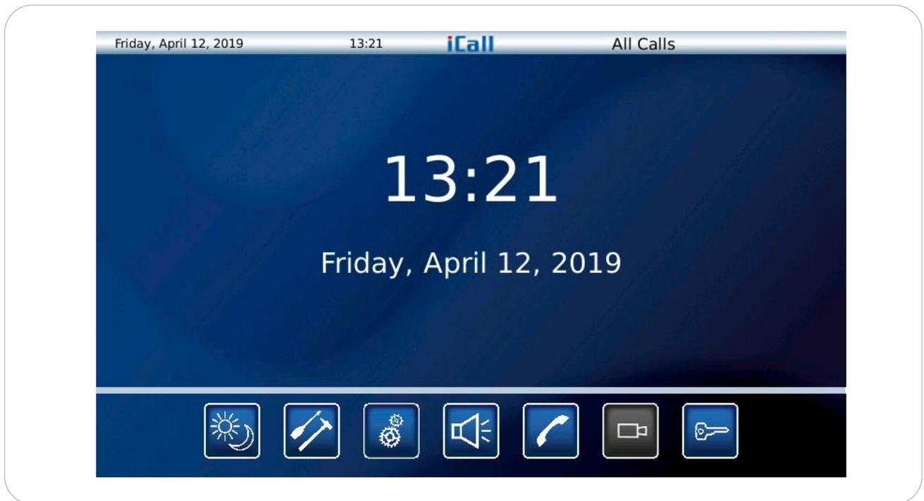
In the idle screen, where no calls are active date and time indication is showed. In the left top corner there is also a date and time indication, this indication is also present if there are active calls on the screen. In the right top corner is an indication on which day/night profile is active. This profile can be change time based or manually by the user.
