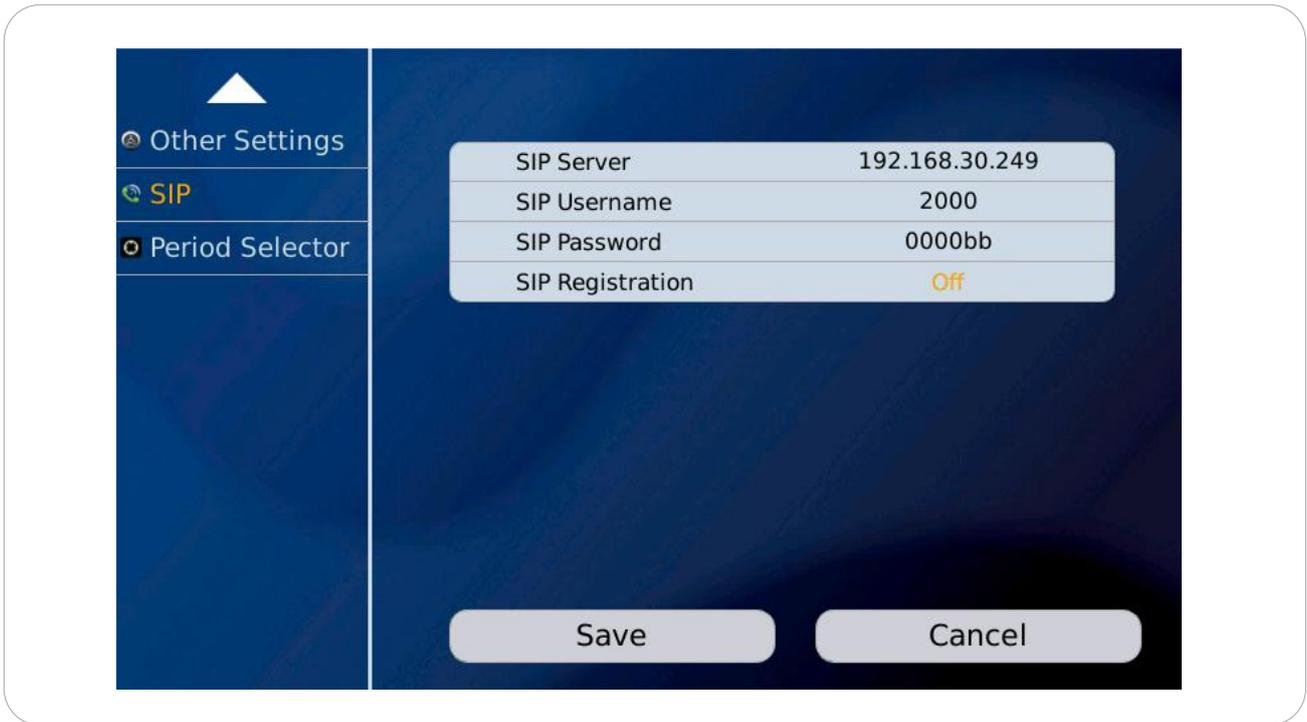
The following parameters can be set up in the SIP settings page:
