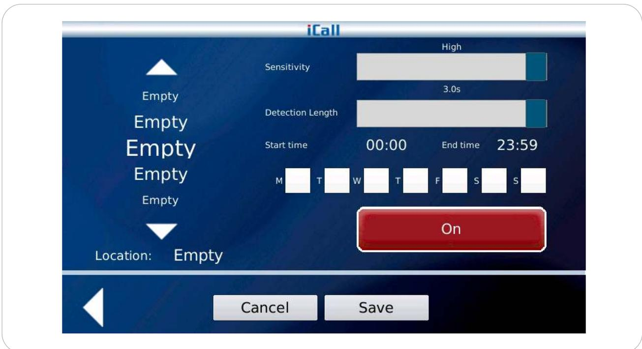
The nurse station can be used for programming acoustic alarm call stations. The sensitivity and length of the acoustic trigger can be set together with the start time and end time and the day of the week the acoustic unit has to function. By pressing the on button the system will set it in service.
