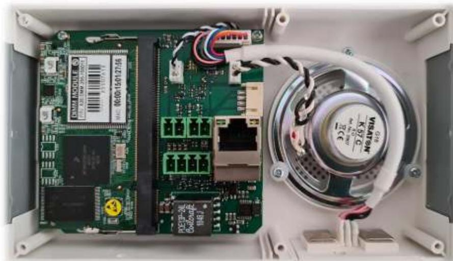
To remove the COM board from the motherboard the latches on the side need to be moved aside and the board removed from the connector at an angle. To place the daughter card back in the motherboard it must be slid into the connector at an angle of approximately 45° and pushed down.
