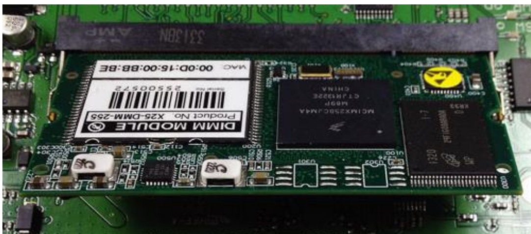
Figure 7: Locking COM module in to DIMM connector
