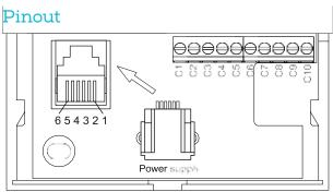
The power supply RJ12 connector is provided to plug in the optional external power supply unit. It could also be used for alternative connectivity, as in the following table.
