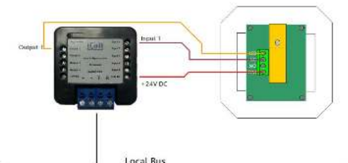
Connecting Normal Closed contact to IO station
