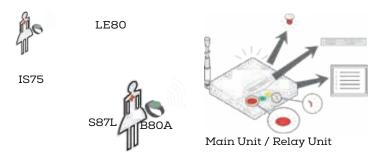
The B80A Wristband Transmitter offers IP67 waterproof protection and has built-in automatic battery monitoring with low battery warning. To communicate correct functioning, it sends an automatic daily radio message to the receiver over radio monitoring.
