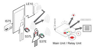
The S37E Wristband Transmitter with Accompany function is built to interact with the following devices:
