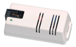
The IS75 Person Detection Beacon is designed to allow the locating of any person wearing a S37L Wristband Transmitter with Locating function in the nearby vicinity. It generates a coded magnetic field which can be identified by the S37L Wristband Transmitter with Locating function. This system may be used to locate patients suffering from Dementia and
