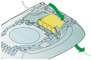
3. Feed the antenna cable through the back of the Carephone, on the right-hand side of the battery pack.
