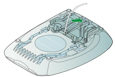
7. Fasten the antenna cable carefully into the channel provided in the middle of the battery pack cover and close the battery pack cover.
