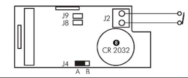
Configuration and wiring must be done before placing the battery in the battery holder.
