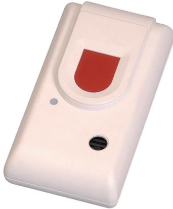
The ManDown Sensor has a built-in tilt device, which can detect if the person holding it is in a horizontal position, such as lying on the floor. The sensor will automatically send an alarm when its position corresponds to horizontality after a certain time. The ManDown Sensor can be held, for example, as a necklace by an elderly person or as a safety device by a lone worker in a hazardous environment. The ManDown Sensor is part of a wireless NurseCall system.
