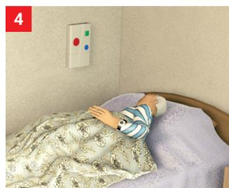
**4** Patients can call for immediate attention by pushing the button on the wrist transmitter. The batteries status is monitored and it is easy to replace the battery, which minimizes maintenance costs and time.
